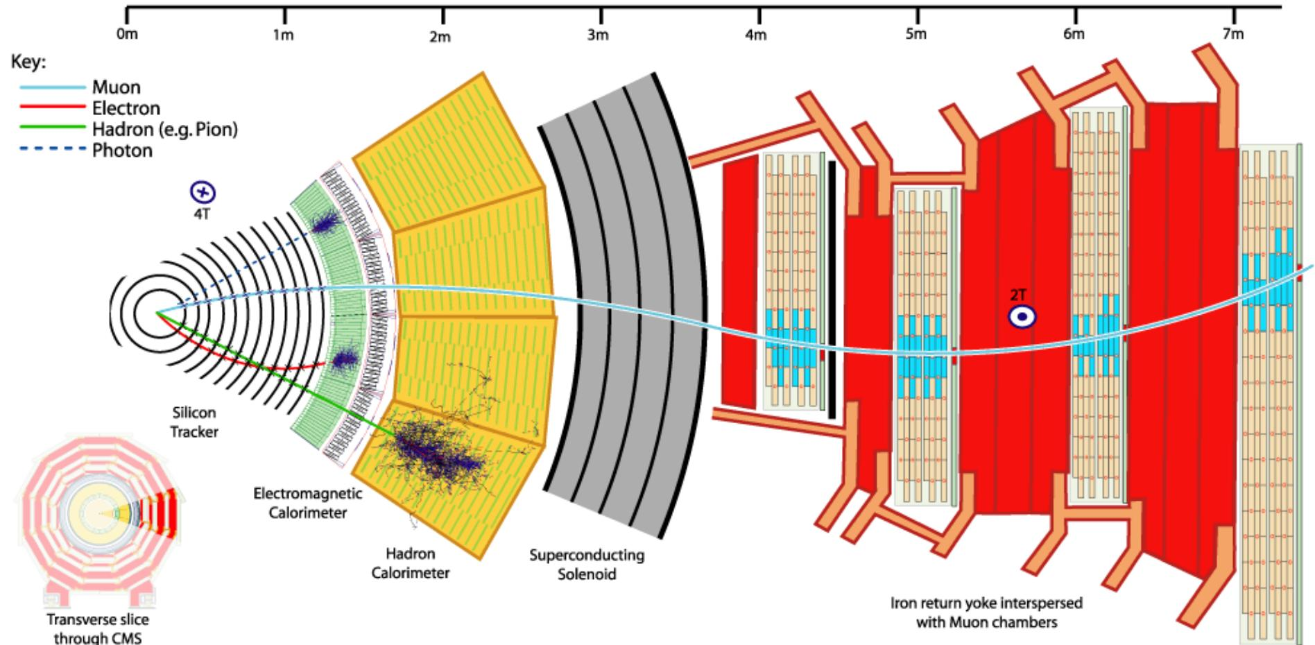
Deflection  $\sim BL^2/p \rightarrow$  need high B (s.c.) and large magnets; need high resolution position measurements ( $10-100\mu$ ) at large  $p$ ; also energy and position measurement thru total absorption (photon, electron, hadron)
