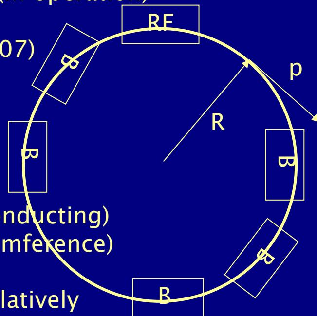
So: need high  $B$  (state of the art magnets, superconducting) and large  $R$  (a circular tunnel with a large circumference)
